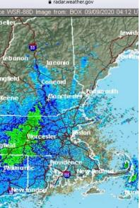
coast line in the "clouds" mirror imaged due to how the tropo layer reflects the radar downwards and the different reflections back if the beam hit the ocean or land.
